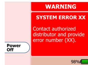
The system error screen is the most general form of error. Also, the Indicator LED on the front of the pump will change to a “Red” status. As seen above, the screen will turn red when this error occurs. **Note: The only way to exit from a System Error is to power down.** An error number is displayed on the screen, for reference purposes. This number should be used when calling Customer Service.
