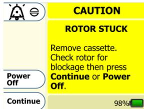
The **ROTOR STUCK** error screen appears when the pump detects an unusual amount of resistance to the rotation of the rotor. (The rotor is the black circular wheel attached to the motor that rotates to move fluid through the feeding set). This error is typically attributed to formula or contaminant build-up on the rotor shaft, which can be corrected by cleaning the rotor. In rare circumstances, this problem could be due to a faulty motor/gearbox assembly.
