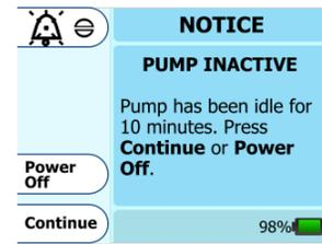
The pump inactive error screen will appear if the pump has been without input for more than 10 minutes.
