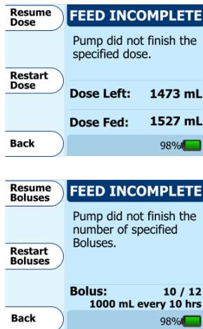
The **FEED INCOMPLETE** screen will appear if a **Dose** or **Bolus** feeding is interrupted prior to completion of the allocated amount. In the pictures, you will see two different screens that may appear in this case. The screen on the top shows an Incomplete Dose. The screen on the bottom shows an Incomplete Bolus.
