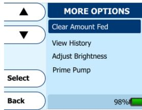
To access the features of **Clear Amount Fed**, **Airplane Mode**, **View History**, **Adjust Brightness**, or **Prime Pump**, press the **More Options** button. Use the arrow keys to highlight the feature you want to activate. Once highlighted, press the **Select** button to activate the highlighted feature. Hit the **Back** button to resume feeding.
