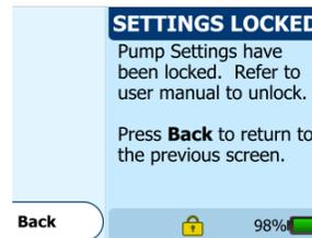
The **SETTINGS LOCKED** screen will appear if the **Lock Settings** feature has been activated in the **Biotech** Mode. By design, no settings can be changed while the pump is in this state. To disable the **Lock Settings**, you must disable this feature in the **Biotech mode**.
