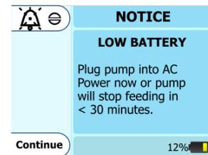
The **LOW BATTERY** screen appears and the alarm beeps continuously when the battery needs to be recharged. There is approximately 30 minutes of battery life remaining when this screen appears
