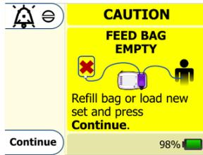
The **FEED BAG EMPTY** screen appears when the enteral formula is no longer being delivered because the bag is empty. Large amounts of foam or bubbles in the feeding solution can also be a cause for this alarm. Check the bag to see if it is empty and re-fill the bag as required. If the bag still contains feeding solution, remove cassette and check the bag side tubing for excessive foam or bubbles. Clear bubbles from line and reload the feeding set or replace with a new feeding set.
