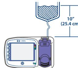
Hang the feeding set bag or fluid container so the starting volume of fluid is 10" (25.4 cm) above the top of the pump as shown.
