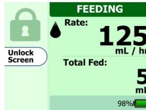
Once activated, a Lock symbol will appear on the **Feeding** screen, showing that the buttons are disabled.
