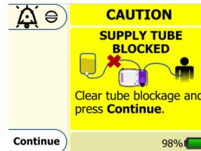
The **SUPPLY TUBE BLOCKED** screen will appear if there is a blockage, obstruction, or kinked tubing between the feeding bag and the pump. Check the tubing between the bag and the pump to see if cause of the blockage can be located and cleared. If the error cannot be fixed, remove the blocked pump set and load a new pump set onto the pump.
