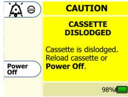
The **CASSETTE DISLODGED** screen will appear if the magnet in the cassette is not properly loaded in the pump set loading area. Reload the cassette to ensure the correct positioning of the cassette on the pump. Check the cassette to see if the black magnet is missing from the cassette. If the error cannot be resolved, load a new pump set, prime it, and press Continue to restart the feeding.
