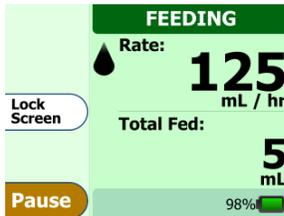
To use the **Lock Screen** option, press and hold the **Lock Screen** button for 5 seconds. A countdown will appear to show how long to hold the button.
