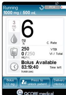
The pump can be unlocked with any code level, functions will be limited according to the code level entered. When Auto Patient Lockout is enabled, Patient Lockout will be reactivated within 30 seconds.
