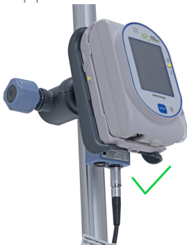
Figure 2.18. Charging Sapphire Connect through Mini-Cradle
