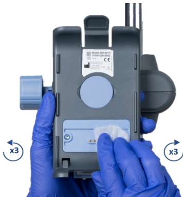
Figure 11.1. Cleaning Electric Connectors
