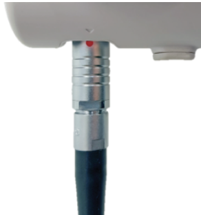
Figure 2.27. Connecting Blue-Buttoned Bolus Handle
