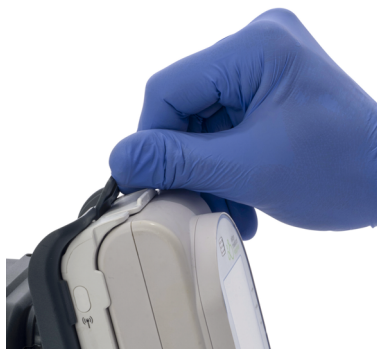
Figure 2.23. Disconnecting from Mini Cradle
