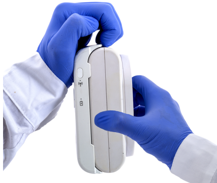
Figure 2.21. Releasing Sapphire Connect from Sapphire Pump
